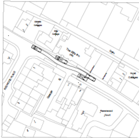
Rigid Vehicle Tracking Plan : Option 3 scale 1:500 @ A1
