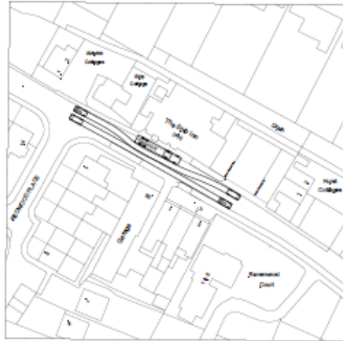
Articulated Vehicle Tracking Plan : Option 3 scale 1:500 @ A1
