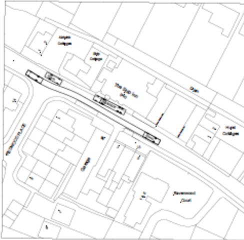
Articulated Vehicle Tracking Plan : Option 2 scale 1:500 @ A1
